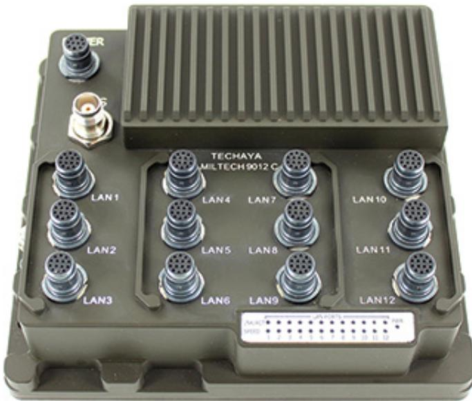
The shrinking of components and platforms has allowed the consolidation of multiple platforms. The Techaya MILTECH 9012X contains an Ethernet switch, an embedded single-board computer, and a GPS receiver.
